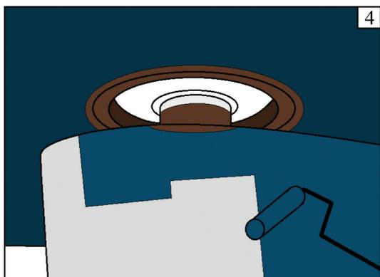
You can now proceed with the antifouling of the hull and rudder blade. Be very careful to not cover any previously antifouled metals and make sure there is absolutely no contact between the antifouling of the hull and rudder blade. **Remember 3-5cm of space between any metal parts from the antifouling!**
